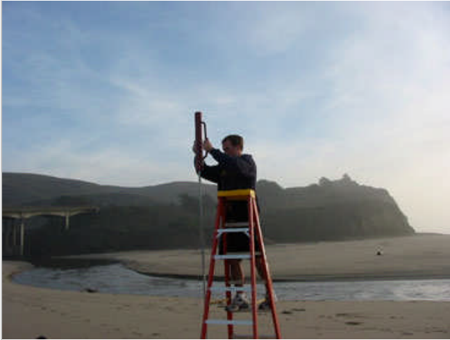
Stanford graduate student Nick de Sieyes installs a monitoring well at a Northern California beach. Credit: Stanford/Kevan Yamahara
