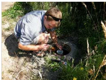
Stanford graduate student Nick de Sieyes deploys a data logger in a monitoring well at the field site in Northern California. Credit: Stanford/Kevan Yamahara
