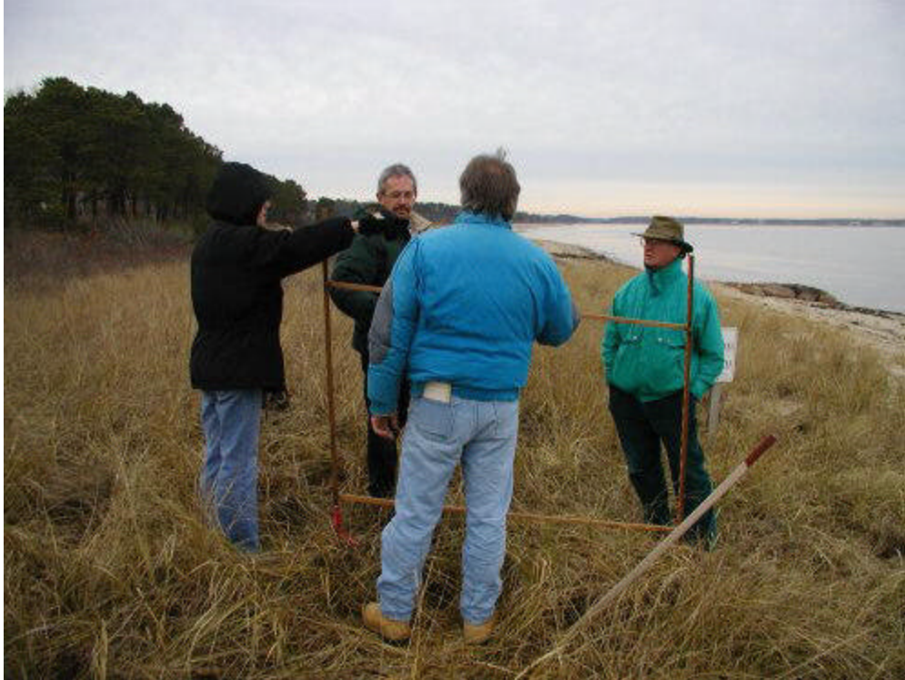
Jim O'Connell (back to the camera) trains volunteers in the Emory Rod Method of dune and beach profiling.
