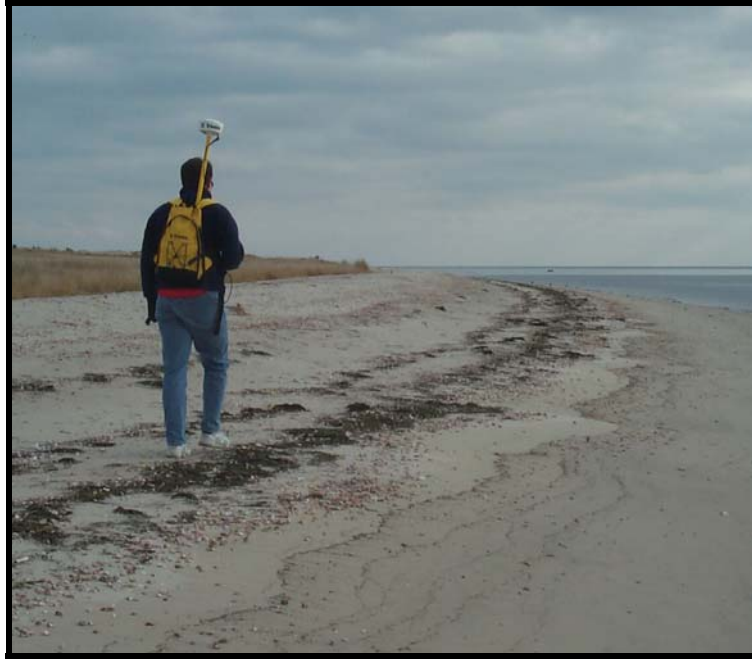
Figure 3. Collecting Dead Neck shoreline position data using a Trimble Backpack DGPS unit.
