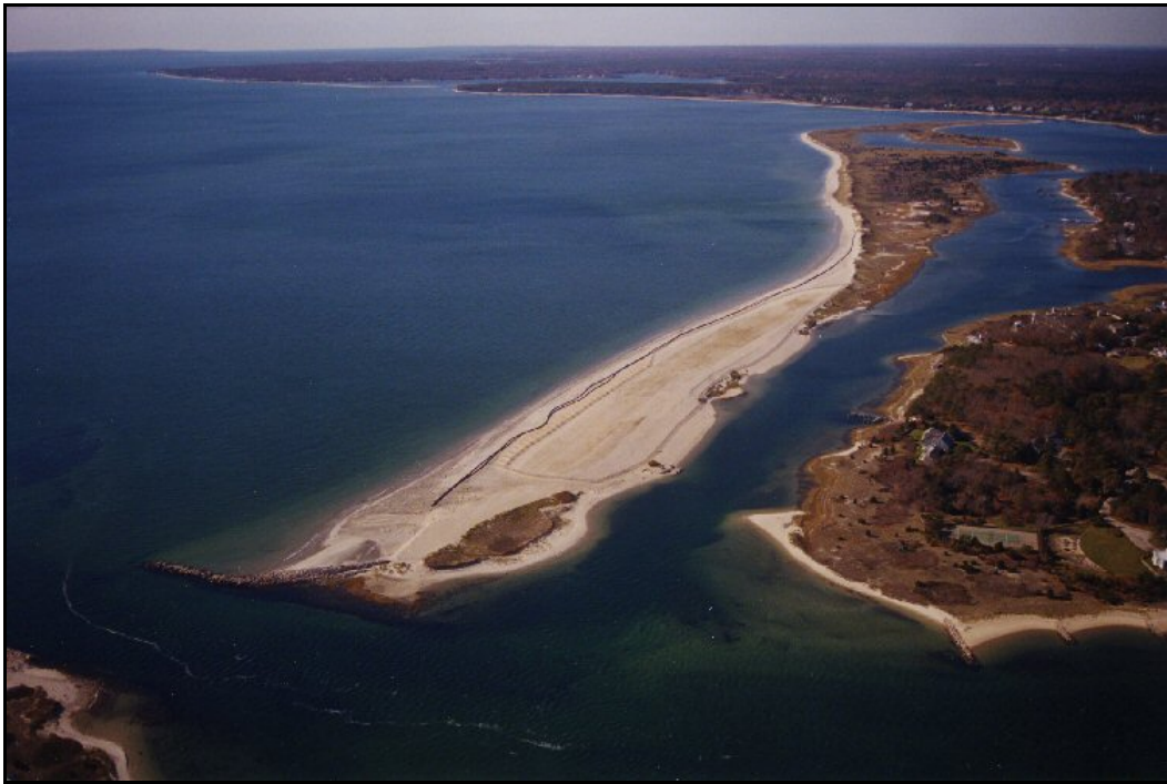
Figure 2. Dead Neck Beach immediately following the beach nourishment in 2000, where the beach width had been increased significantly to prevent breaching of the barrier.
