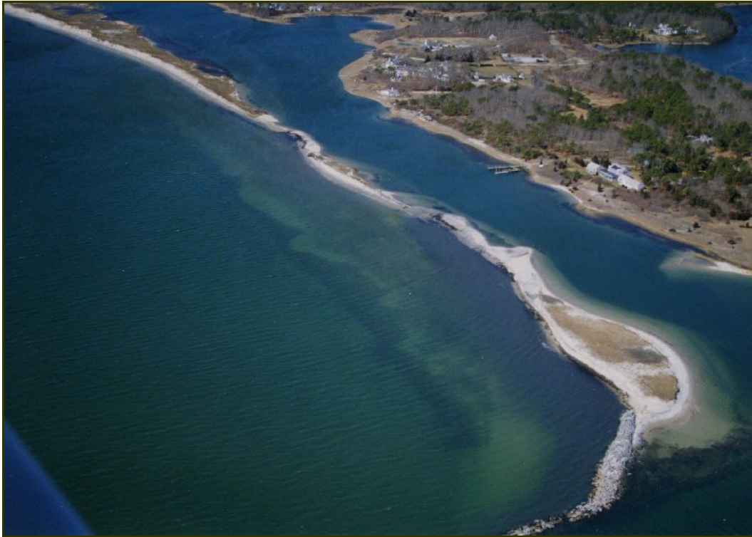
Figure 1. The eastern portion of Dead Neck in 1999, showing at least two locations where the beach had significant storm overwash areas.
