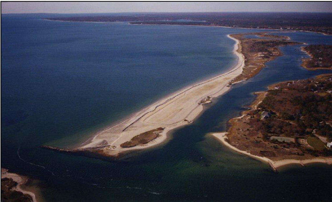
Figure 5. Dead Neck Beach immediately following the beach nourishment in 2000, where the beach width had been increased significantly to prevent breaching of the barrier.
