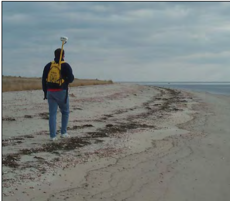
Figure 1. Collecting Dead Neck shoreline position data using a Trimble Backpack DGPS unit.
